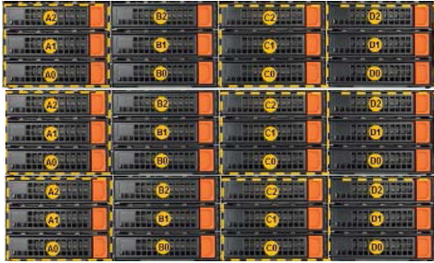
Figure 3. ASU-100E “Minimum” configuration of three “Smart” enclosures.
