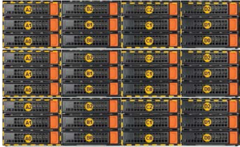
Figure 3. ASU-100E “Minimum” configuration of three “Smart” enclosures.
