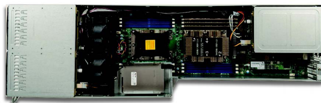
Figure 2. ASU-100XL storage node top view.
