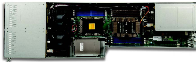
Figure 2. ASU-100XL storage node top view.
