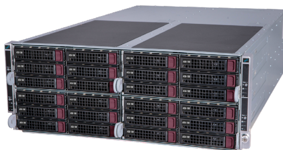
Figure 1. ASU-100 enclosure with four storage nodes.
