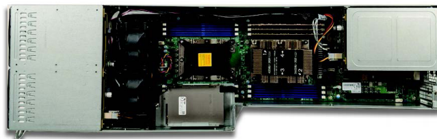
Figure 2. ASU-100 storage node top view.
